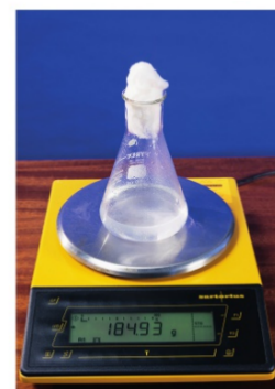
▲ fig C Cotton wool is placed in the neck of the flask to prevent the loss of liquid spray.
